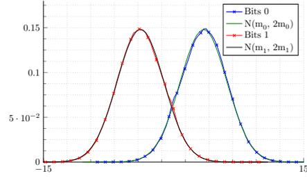
Fig. 1: Probability density function of the LLRs at the output of GSM GMSK decoder vs symmetric Gaussian distribution when a priori mutual information is 0.5.  $m_0$  (resp.  $m_1$ ) is the expected value of LLRs associated with bits 0 (resp. 1).
